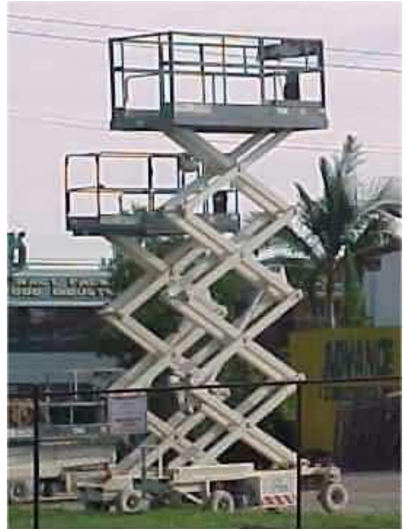
Perancah udara (Aerial Scaffolding)
